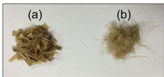
Figure 16. Pictures of the chopped flax fibers: (a) silanized and polymer-coated and (b) silanized. [Color figure can be viewed in the online issue, which is available at wileyonlinelibrary.com .]
